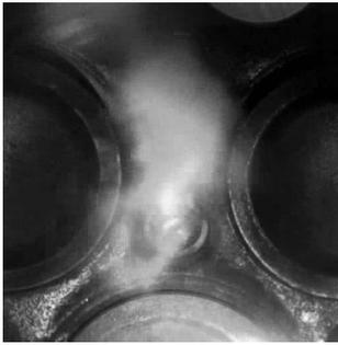
Figure 13. Slight fuel impingement on intake valves due to larger spray angle
