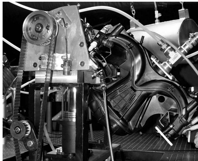
Figure 7. View of the single cylinder optical engine
